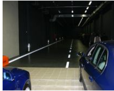
In more than 50m long light tunnel, which fulfils all the parameters of main road, developers review headlights of prototypes and take photometric and colorimetric measurements.
