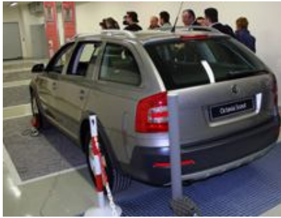
Development and testing of the electronic parking sensors, which work on the base of ultra-sound, proceed in a special room with a number of road surfaces.
