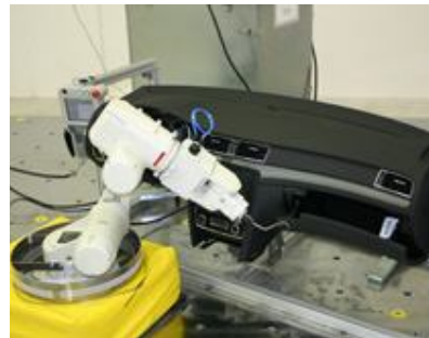
The tireless robot takes care of long-time checking of quality, function and reliability of controls on the dashboard..
